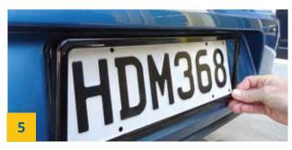
Attach the frame by starting at the bottom. Clip it securely into place .
