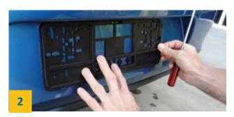
Choose a hole combination on the base plate which is suitable for your car
