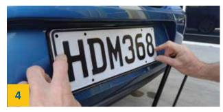
Place the number plate centrally on the base plate and ensure that it is held by all the plates retainers
