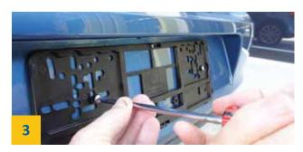
Fix the base plate to the car with the included washers and suitable screws
